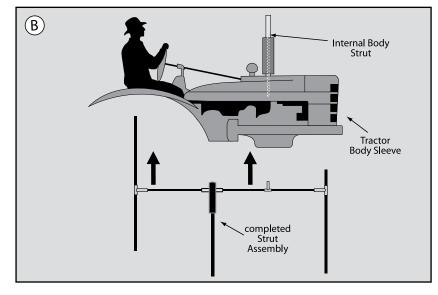
The Strut Assembly of your Tractor spinner is shipped in three sections. Connect Center Rods of the Rear Strut Assembly and the Front Strut Assembly to the Center Rod of the Center Strut Assembly as shown. (diagram A)
