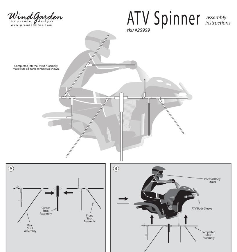
**Step 1**The Strut Assembly of your ATV spinner is shipped in three sections. Connect Center Rods of the Rear Strut Assembly and the Front Strut Assembly to the Center Rod of the Center Strut Assembly as shown. (diagram A)
