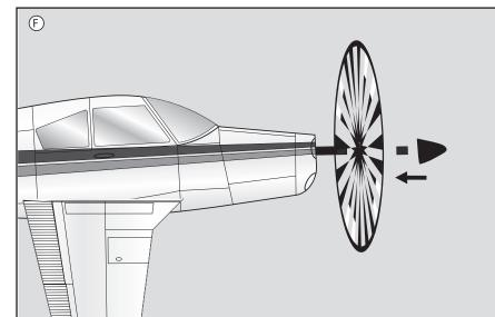
Remove the white, wooden end cap and spacer from the propeller axle exiting from the front end of the fuselage. Slide on the Spinner Propeller. Place the Spinner Propeller onto the propeller axle, then replace the spacer and the end cap. (diagram F)
