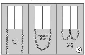
Tail loop inside. The Fuzzi Tail can be attached in different ways depending on amount of drag desired as shown in diagram B.
