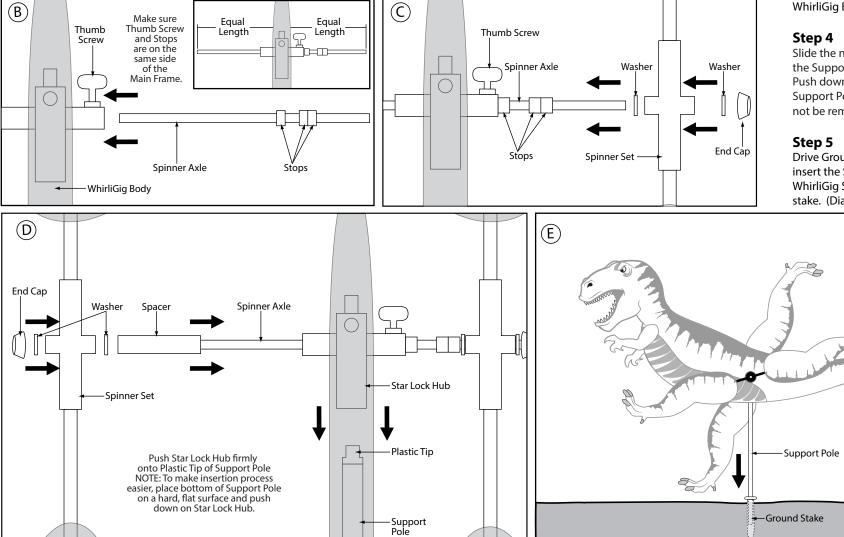
spinner set aside. Slide one Washer onto the side of the Axle with the Stops. Decide which way you want the arms or wings to face and slide one set onto the Axle followed by the remaining Washer. Carefully pound the End Cap onto the Axle. Repeat with the remaining parts on the other side of the Axle, making sure to place the Spacer closest to the WhirliGig Body. (Diagrams C & D)
